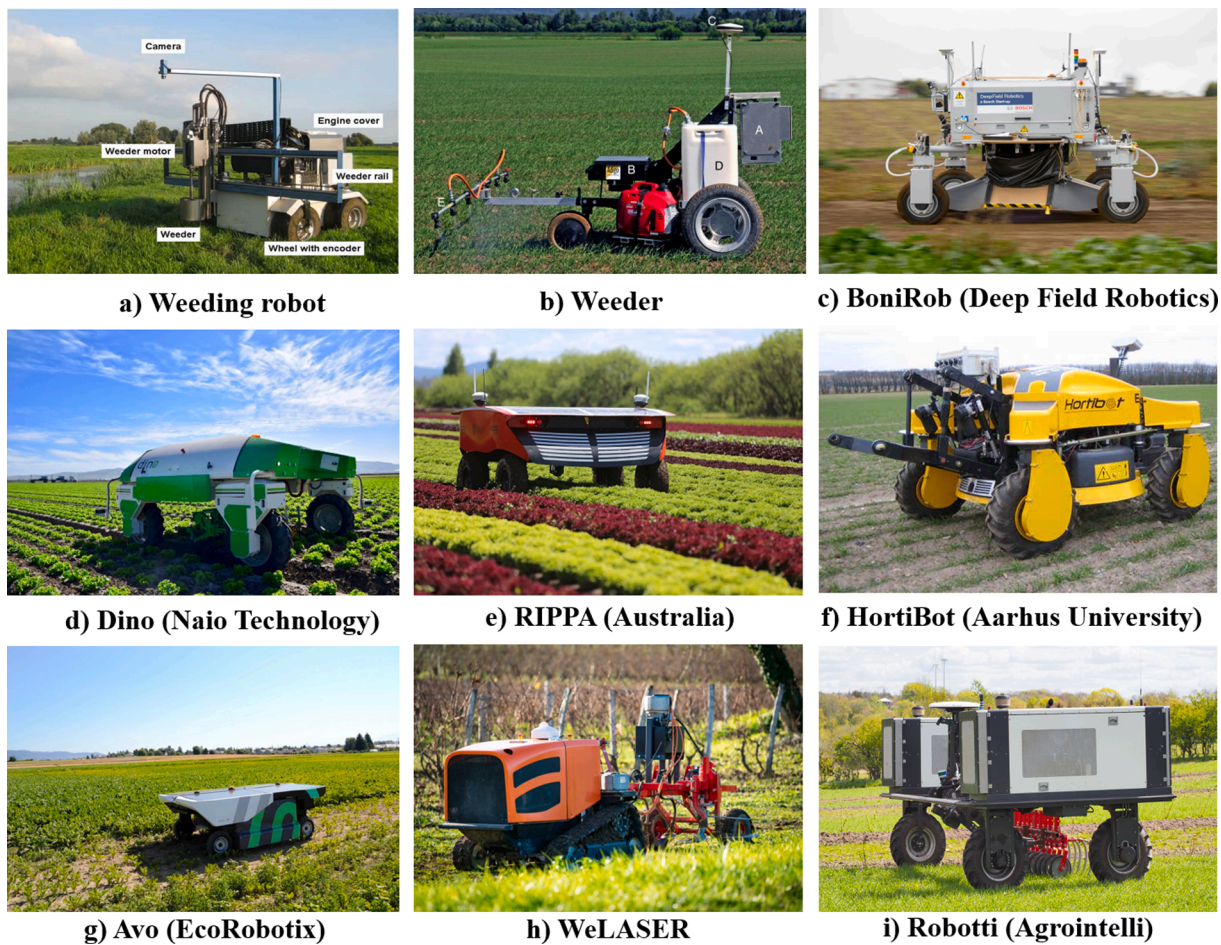
Fig. 6. Commercial robots that use computer vision techniques to perform in-field weeding tasks.
