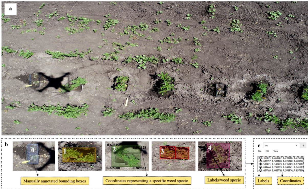
Fig. 6. Manual annotation of the image data consists of three steps, (a) acquiring the aerial image, (b) manually annotating each class of weed species, and (c) exporting a text file consisting of labels and coordinates.
